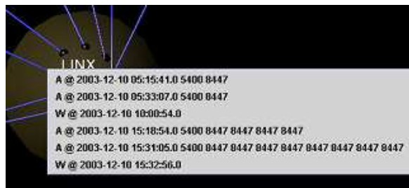
Figure 5: Example for “BGP-4 Update” Pattern describing the “manual trial-and-error to traffic engineering operations” heuristics
